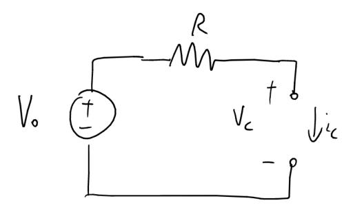
Obviously, the current \$i\_C\$ is going to be zero. And because there's no current going through the resistor \$R\$, \$v C\$ equals \$V 0\$.
