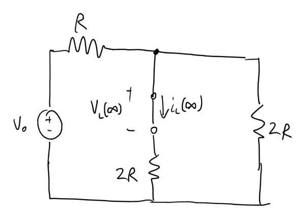
Obviously, the voltage across the inductor  $v_L(\inf y) = 0$ . Current can be solved by whatever circuit analysis technique you prefer, and it comes out to  $i_L(\inf y) = \frac{V_0}{4R}$ .
