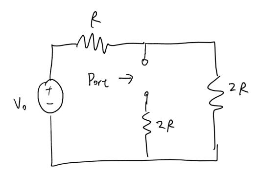
Since we're calculating Thevenin resistance, we can turn off the independent source  $V_0$ . Then  $R \{TH\} = 2R + R // 2R = \frac{8R}{3}$ \$.
